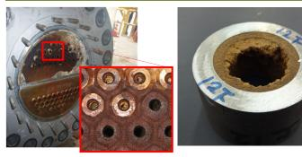
Produced waters and waste waters experience various changes in temperature and pressure. Such changes cause the precipitation of minerals (scale), and these minerals can clog tubing in wells or pipes in facilities.
