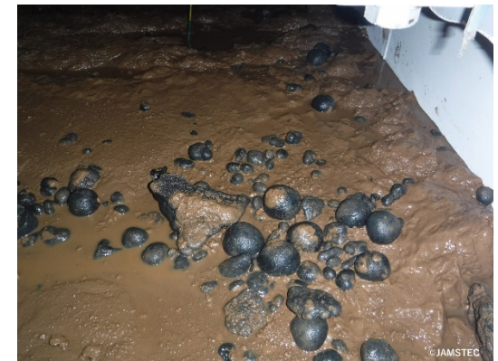
Collected deposit samples with pellets of polymetallic nodules at sea bottom of deeper than 5,000m water depth
