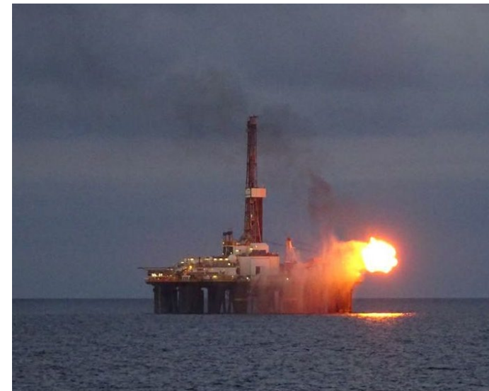
Production test at the Seagull Block
