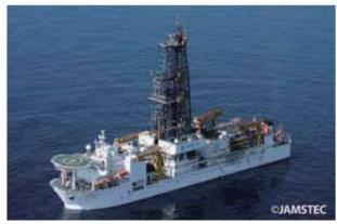
The CHIKYU, the scientific drilling ship used in the first production tests
