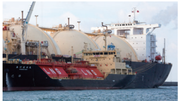
LNG being transferred from an ocean-going LNG vessel (background) to the domestic LNG vessel Akebono Maru (foreground)
