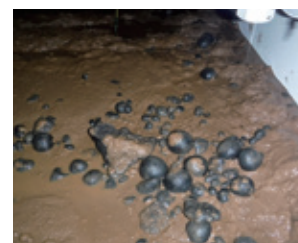
Collected sediment samples in EEZ waters around Minamitori-shima Island (spherical materials are manganese nodules containing copper and nickel).
