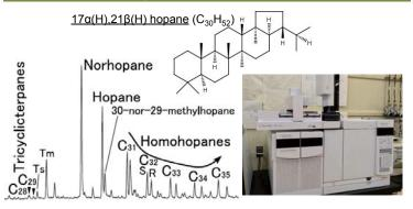
To separate and identify various compounds, such as biomarkers in crude oils, gas chromatography-mass spectrometry (GC-MS) is used. Various compounds are separated by GC based on differences in their boiling points and then identified according to the mass spectra specific to individual compounds using MS.
