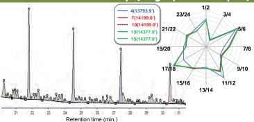
Chemical compositions of crude oils differ slightly between each reservoir, even if the source of two reservoirs is the same. These slight differences can be evaluated through fingerprint analysis using GC chromatograms. Fingerprint analyses are applied in reservoir continuity and connectivity studies as well as production allocation studies of different reservoirs.
