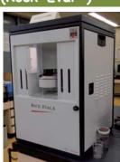
Gas-prone Rock-Eval® is a unique instrument used in the petroleum industry. The organic types (oil-prone or gas-prone) and maturity of source rocks can be estimated using Rock-Eval® pyrolysis.
