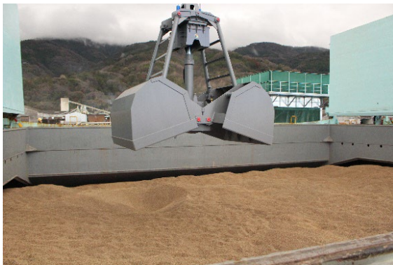
Unloading wood pellets from a ship
